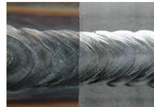
Laser Rust Removal
